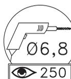
This symbol shows the drill diameter in millimetres and refers to drawing 250, which shows the correct method of drilling holes for steel components. Metal filings must always be cleared away to prevent rusting.
